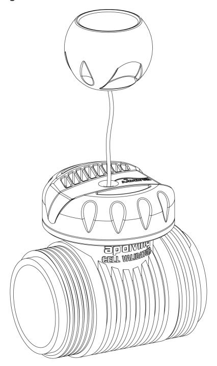
The cell validator has two different threads on the same moulding for complete compatibility with all AP rebreathers produced since January 2003.
